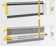
Measure from floor to the top of the existing back plate.
