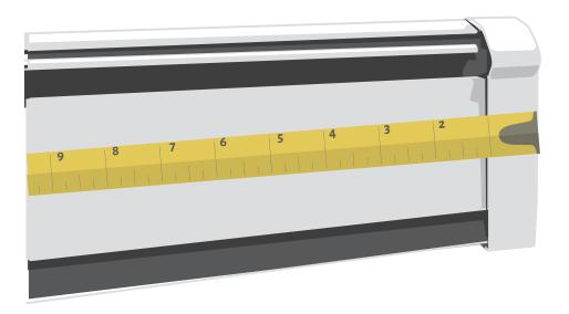
Measure from one end of your baseboard heater to the other end. If a straight section is missing the back plate, measure from one extreme end of desired coverage to the other extreme end of coverage. This is the ideal panel length.
