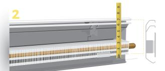
Height from bottom of fin tube to top
