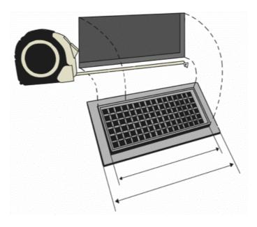
Measure your opening. Use width by height to determine the size of the grille you need, the overall size will be larger when you include the frame.
