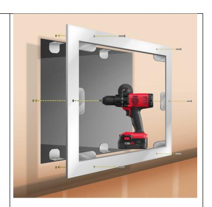
Install your filter so it lays on the filter bracket holders behind the metal strips that are on the frame.
