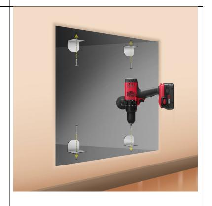
Screw the frame into the wall.
